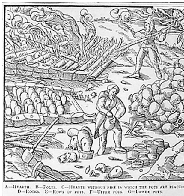
Fig. 18 The production of mercury by downward distillation in the 16th century in central Europe. From [24]
