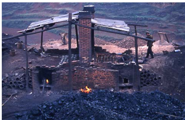
Fig. 10 A typical two-unit smelter near Huize in Yunnan. The fire boxes are on the outside of the retort chamber and with a central chimney. From [9]
