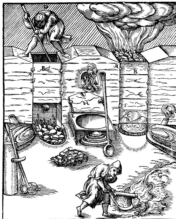
Fig. 2 Workers scrapping zinc oxide off the walls of the silver/lead furnaces at Rammelsberg in the 16th century. From [25]
