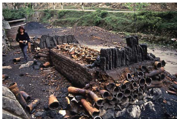
Fig. 8 An abandoned horse trough furnace, probably of the 1980s, photographed in the 1990s, still containing its last load of retorts. From [9]
