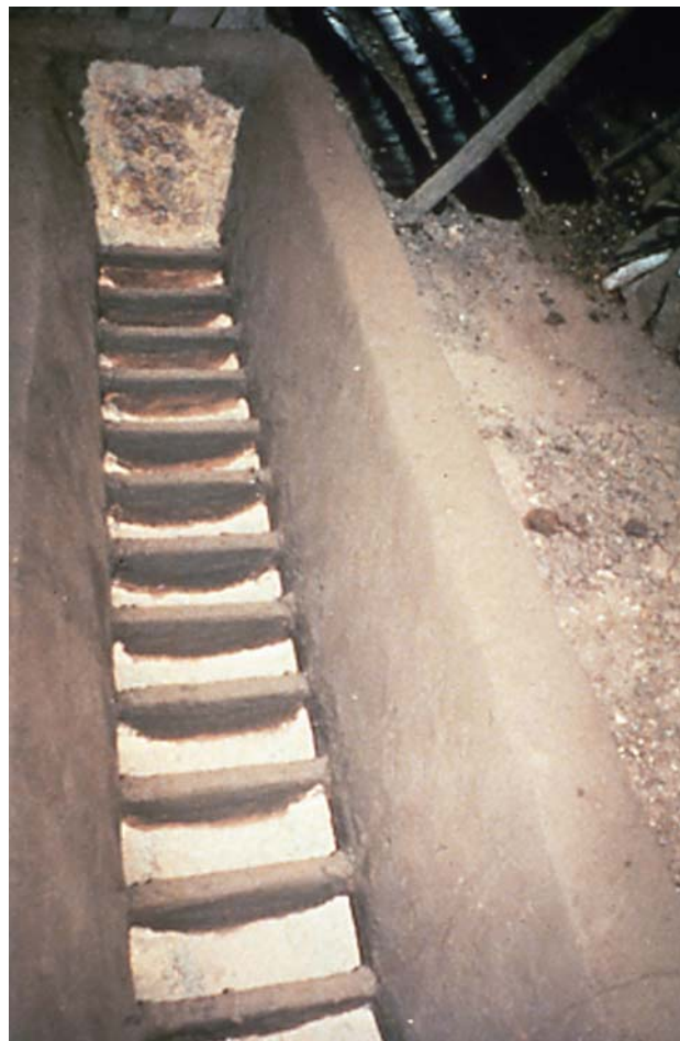
Fig. 7 Empty horse trough type furnace showing the bars on which the retorts will stand. cf Fig. 8. From [13]
